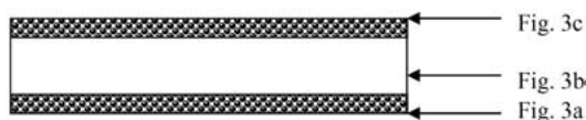
Figure 2 Schematic of the cut Ti sample and the position of the surface observed via SEM.
